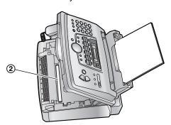
**11** Install the drum and toner unit (1) by holding the tabs.
